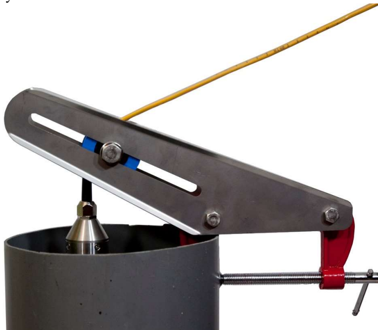
FIGURE 3 - THE POSITION OF THE BLUE PULLEY CAN BE REGULATED
