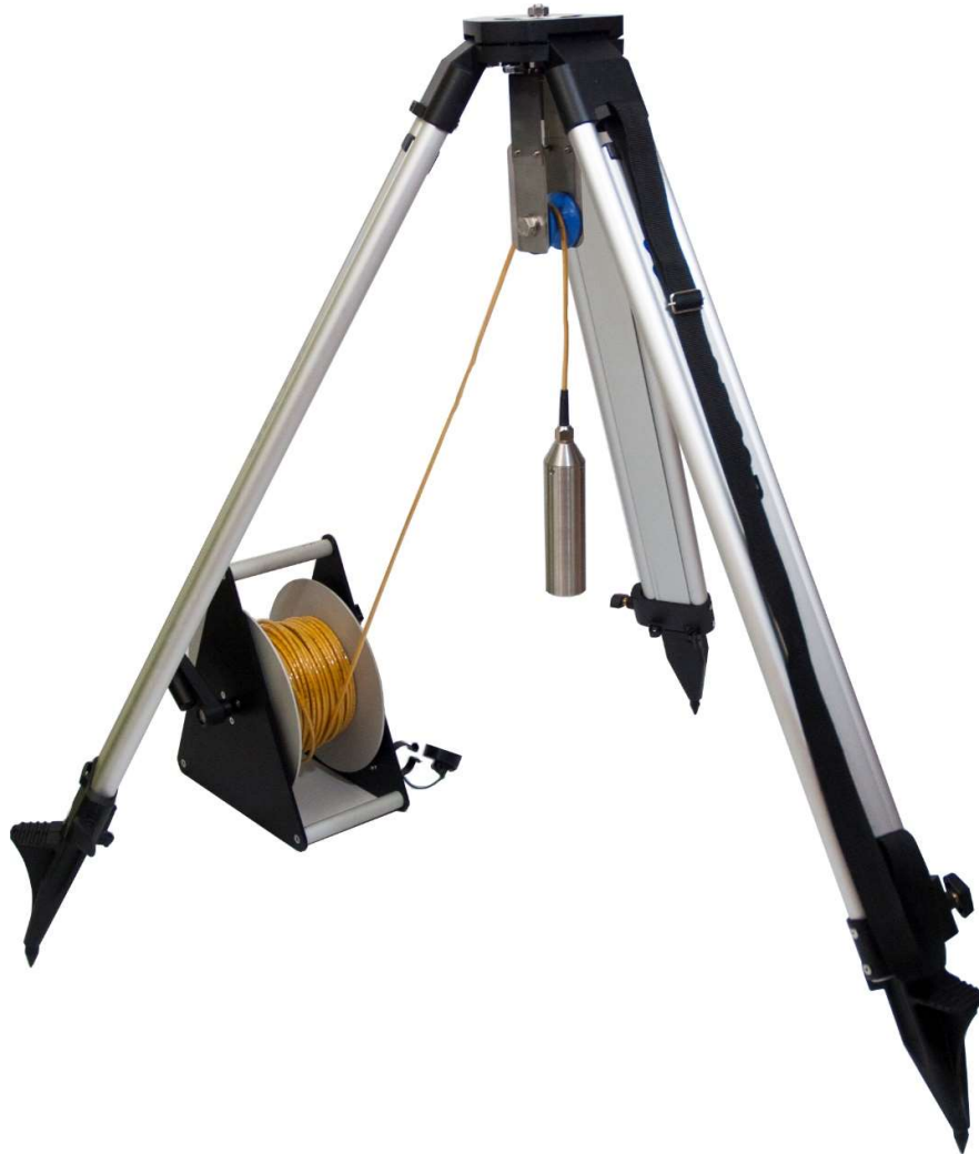
FIGURE 4 - SUSPENDING TRIPOD WITH PULLEY
